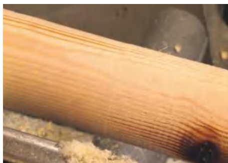
▲ Pic.14 Here you can see the quality of the cut off the skew compared to the spindle roughing gouge. The only time this cut won't work is on really hard, dense woods
